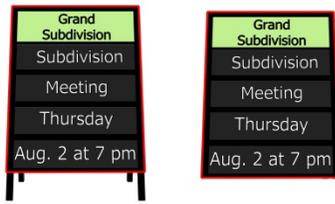
For an A-frame sign, measure sign area by the full extent of the sign and support structure (inside red area), except for legs.
