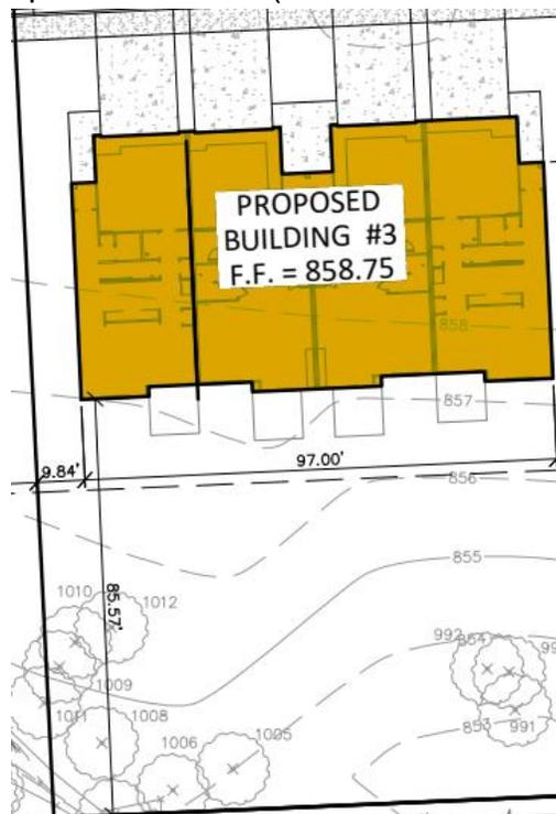
The difference in these setbacks is 85.57 ft – 76.94 ft or a difference of 8.63 ft. Additionally, these setbacks are to the building and not the patio so after taking this into account, the setbacks on the southern perimeter are between 73-76 ft to the property line. This fails to meet the 75 ft bare minimum suggested as a revision to the plan.
