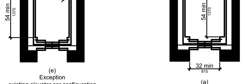
Figure 408.4.1 Limited-Use/Limited-Application (LULA) Elevator Car Dimensions
