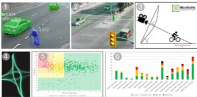
1: AI Detection 2: AI Tracking 3: Monocular Spatial Translation 4: Trajectories 5: Near-Misses 6: Precision Diagnostics
